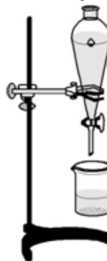
Fig. 2: support and use of the separatory funnel.
